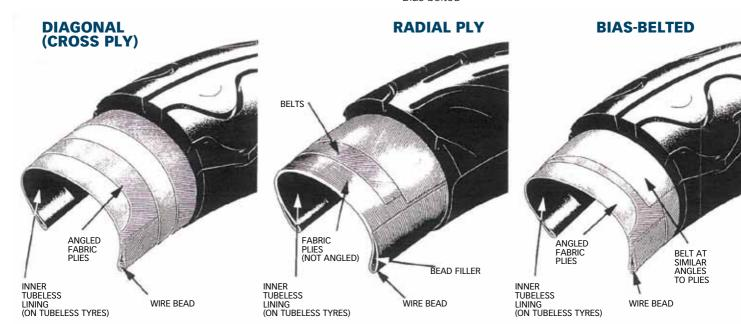
Depending on the wheel type, these may be tubeless (no tube required); or tube type (requiring an inner tube).
